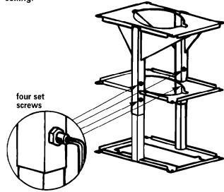
Determine the height of the canopy. The range hood requires at least 24 inches of clearance between bottom of range hood canopy and cooking surface.
